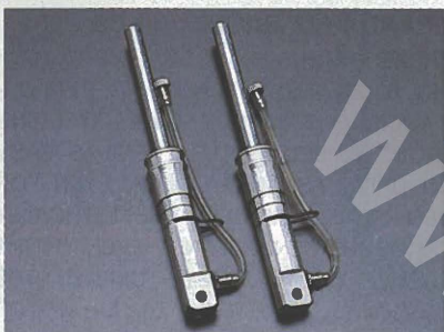
No.GPW-1 OIL-FILLED FRONT FORKS. BETTER CONTROL.
