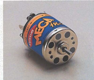
MEGA MOTOR 20x2 ON-ROAD No.2475 20 TURN DOUBLE WIND. IDEAL FOR ANY 1/10 OR 1/12 SCALE ON-ROAD RACING. ALSO SUITABLE FOR 2WD OFF-ROAD RACING. WET-PROCESS MAGNETS FOR EXTRA POWER. 24,000 RPM MAX.
