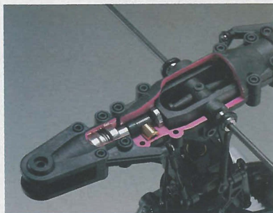
UPGRADED HEAD. NEW ROTOR GRIP. STAINLESS BALL LINKAGES. NEW THRUST BEARING. HARD DAMPER.
