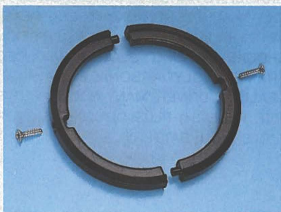
No.GPW-7 LIGHT FRONT WHEEL WEIGHT. FASTER STEERING RESPONSE.
