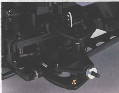
COMPLETELY SCALE DOUBLE-WISHBONE INDEPENDENT FRONT SUSPENSION WITH QUALITY FRICTION SHOCKS.
